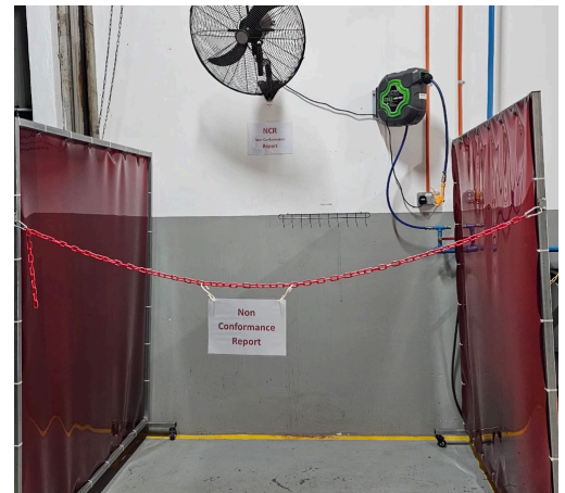
KLH NCR holding area with physical segregation.
